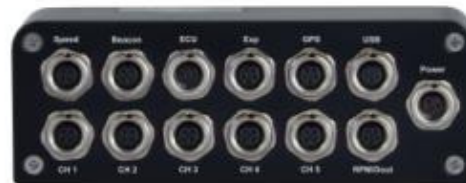
SnoMAX-S 5 Analog Inputs 130x35x47mm, 330g
