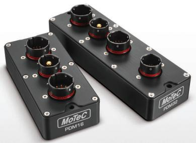
*MoTeC*'s PDM16 and PDM32 Power Distribution Modules replace conventional relays, fuses and circuit breakers by providing electronically switched power to the various electrical systems in the vehicle, including motors, lights, solenoids and electronic devices such as ECUs and data systems. This simplifies wiring and switch requirements, while increasing reliability.
