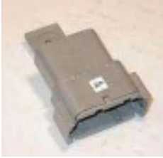
CIM module (computer-interface module) Converts TTL to RS-232 M CIM
