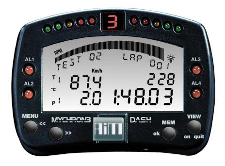
When the session is over it is possible to recall stored data pressing "**MEM/OK**". The display shows test and lap number the data refer to under the RPM Bar graph (in the above image: "TEST 02 – LAP 001").
